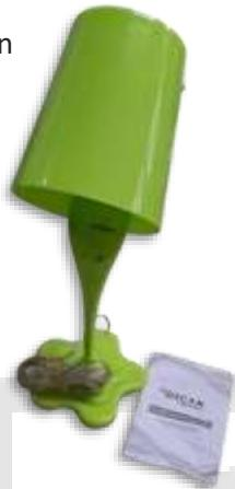
**Child appealing luminaire 3D Space, article number JM2231** poses risk of electric shock and fire because it is improperly designed, i.e. it does not have a protective transformer and the cross-sectional area of the conductors in the supply cable is smaller than the permitted minimum.
